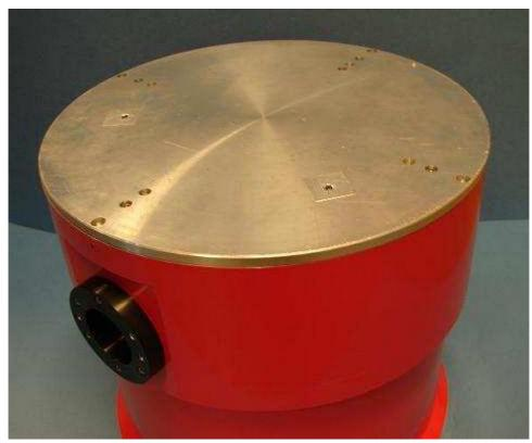
Photo 1.2. Cryostat with transit plate in position
