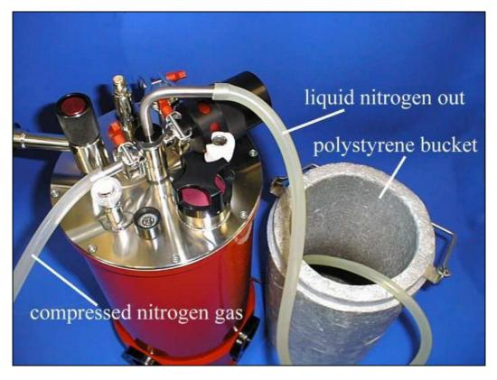
Photo 3.4. Arrangement to blow the liquid nitrogen out of the liquid helium reservoir
