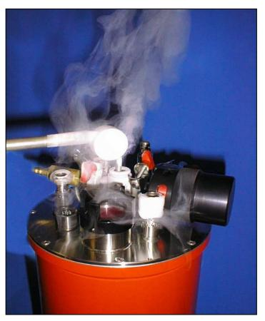
Photo 4.2. Helium gas exhaust during fill
