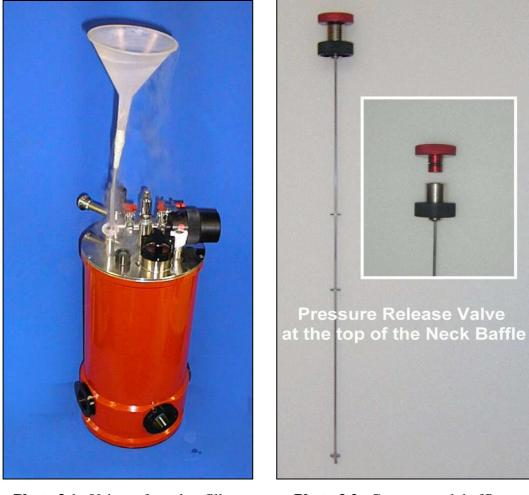
**Photo 3.1.** Using a funnel to fill a cryostat with liquid nitrogen
