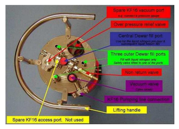
Photo 2.1. Cryostat top-plate fittings
