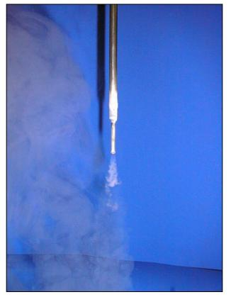
Photo 4.4. liquid helium emerging from a cold tube
