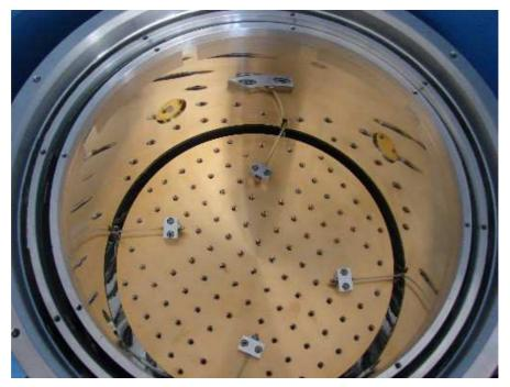
**Photo 1.4.** View inside the cryostat cold space showing the 4.2K cold plate and four support struts
