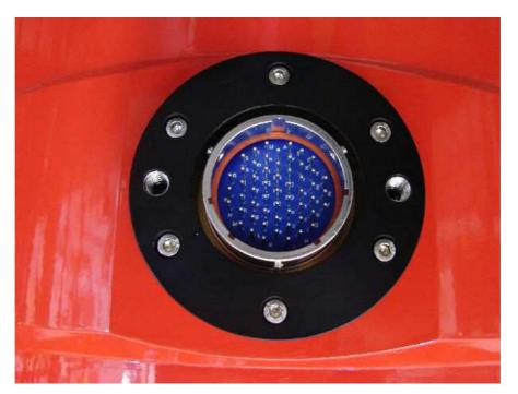
Photo 1.1. Cryostat 55-pin electrical connector
