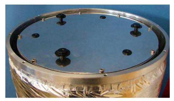
**Photo 1.4.** 77K radiation shield extension mounted on the cryostat along with the 40K gas cooled shield base-plate mounted in position. Note the 3 black nylon spacers used to separate the 4.2K and 40K base-plates, and the 3 black nylon spacers in position for the 77K radiation shield base-plate to be installed.
