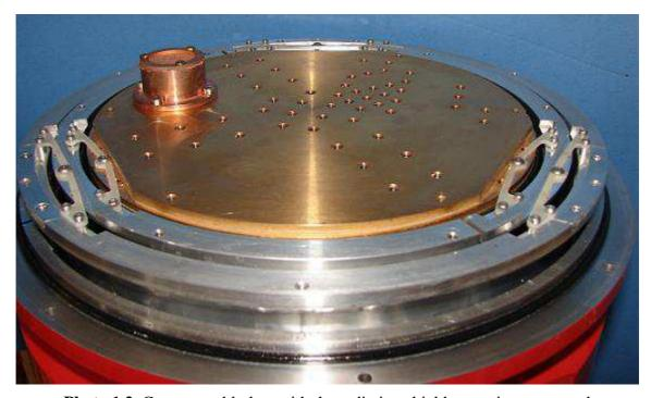
**Photo 1.2.** Cryostat cold plate with the radiation shield extensions removed
