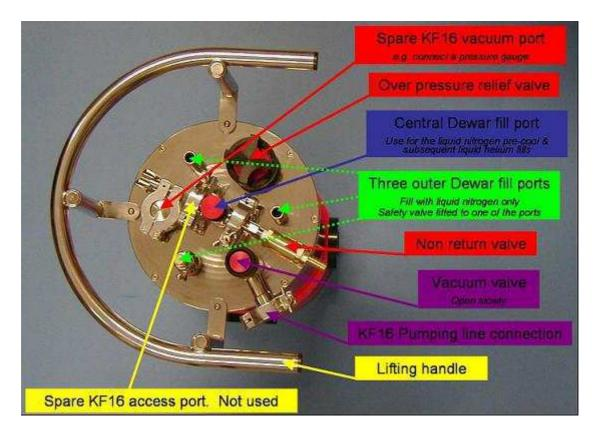
**Photo 2.1.** Cryostat top-plate fittings
