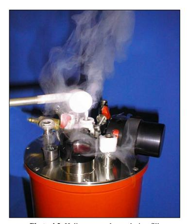
Photo 4.2. Helium gas exhaust during fill
