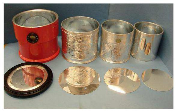
Photo 1.3. Cryostat radiation shield extensions and radiation shield base-plates
