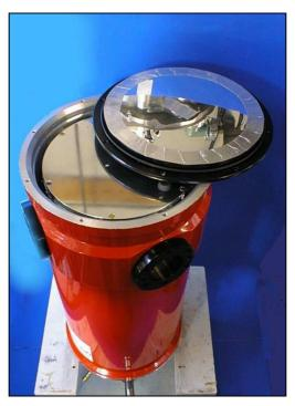
Photo 1.4. Liquid nitrogen base-plate in position
