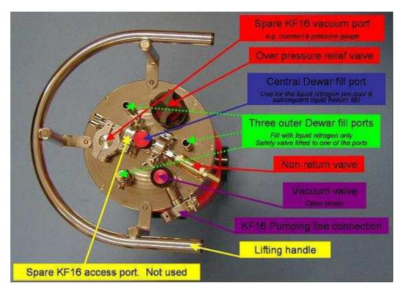
Photo 2.1. Cryostat top-plate fittings
