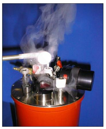
Photo 4.2. Helium gas exhaust during fill
