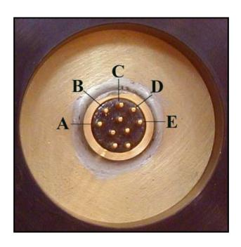
**Photo 4.4.** Electrical port pin assignments. Each of the cryostat's electrical ports are labelled with their respective channel number and pin allocations.
