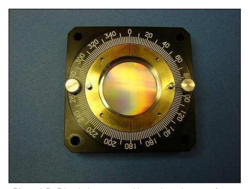
**Photo 1.5.** P2 polariser mounted in graduated support frame
