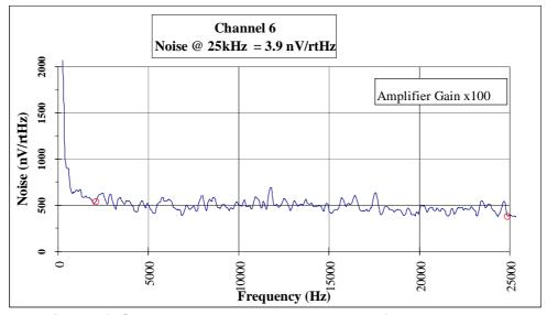
Fig. 6.3f. Channel 6 output noise spectrum from 0 to 25kHz
