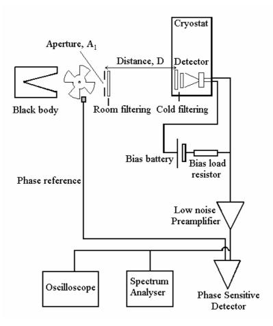
Fig. 6.1. The optical test arrangement
