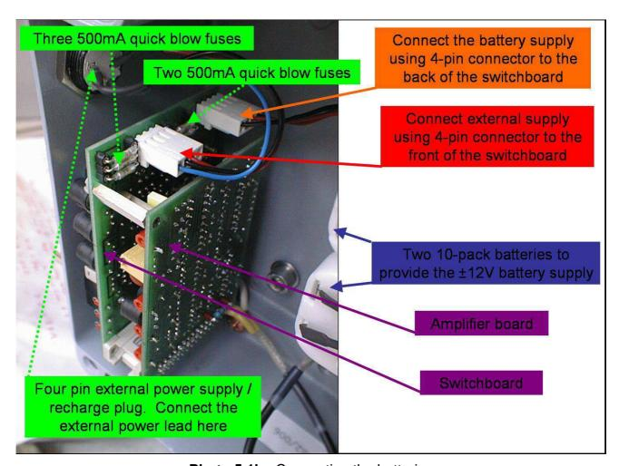
Photo 5.1b. Connecting the batteries
