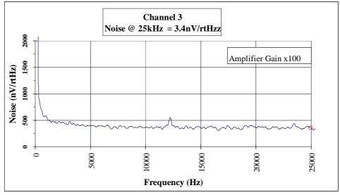
Fig. 6.3c. Channel 3 output noise spectrum from 0 to 25kHz
