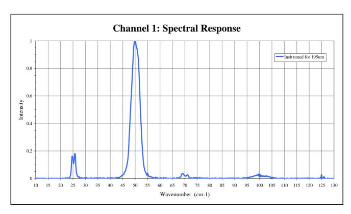
**Fig. A.2.** Measured **s**pectral response of the channel 1 InSb detector with the 100cm<sup>-1</sup> low-pass filter and 195μm band-pass filter in place
