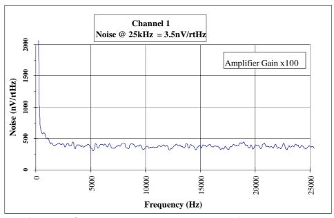
Fig. 6.3a. Channel 1 output noise spectrum from 0 to 25kHz
