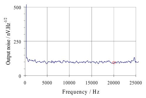
**Fig. 5.1b.** Typical preamplifier input shorted noise spectra Amplifier gain = x100. Noise at  $20kHz = 1.0nV.Hz^{-1/2}$
