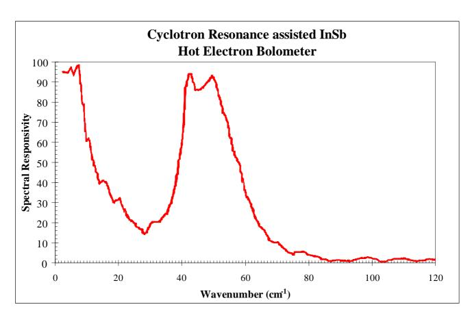
Fig. A.1. Spectral responsivity of a Type QFI/XB detector
