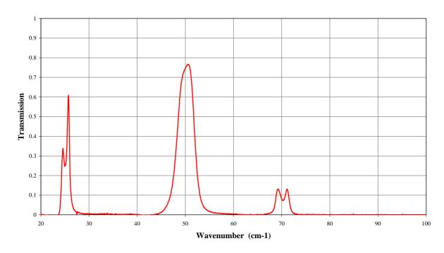
Fig. C2. Transmission spectrum for the type QMMF 195
