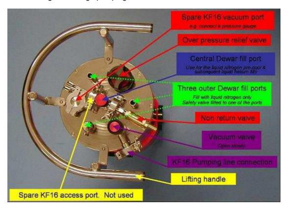
Photo 2.1. Cryostat top-plate fittings
