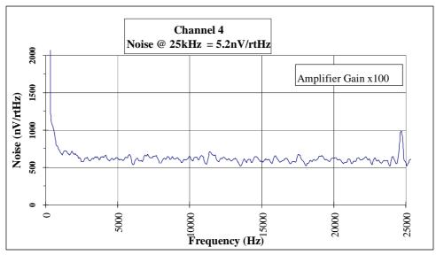
Fig. 6.3d. Channel 4 output noise spectrum from 0 to 25kHz
