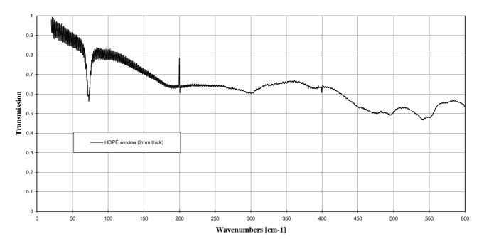
**Fig. C.3.** Measured transmission of a 2mm thick HDPE window from  $20 \text{cm}^{-1}$  to  $600 \text{cm}^{-1}$ . The polyethylene characteristic absorption increase is clearly seen around  $73 \text{cm}^{-1}$
