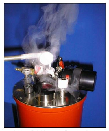
Photo 4.2. Helium gas exhaust during fill
