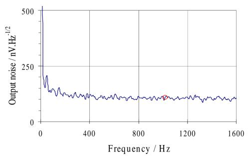
**Fig. 5.1a**. Typical preamplifier input shorted noise spectra Amplifier gain = x100. Noise at  $1kHz = 1.0nV.Hz^{-1/2}$
