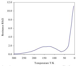
Fig 6.2. Typical resistance versus temperature profile for an InSb detector
