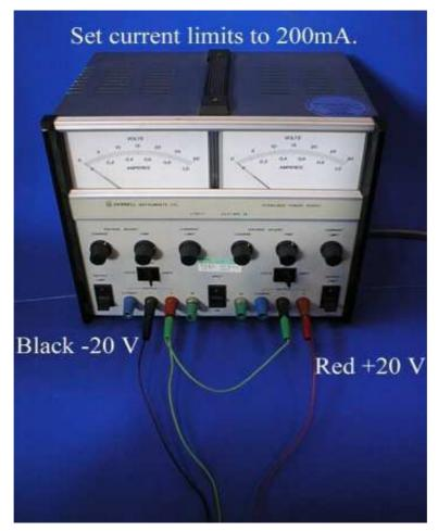
Photo 5.2. Power supply connections
