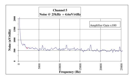
Fig. 6.3e. Channel 5 output noise spectrum from 0 to 25kHz
