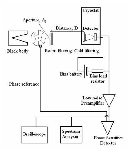
**Fig. 6.1**. The optical test arrangement
