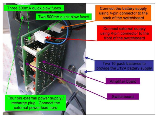
Photo 5.1b. The preamplifier boards
