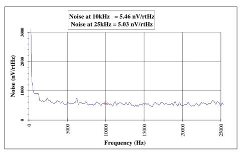
Fig. 6.3b. System output noise spectrum (<25 kHz). x100 gain
