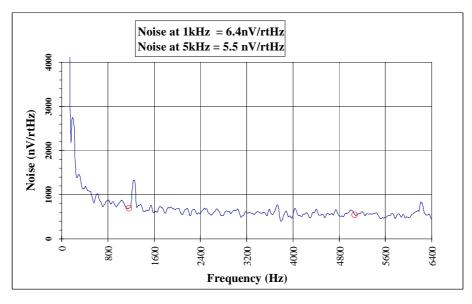
Fig. 6.3a. System output noise spectrum (<6.4 kHz). x100 gain
