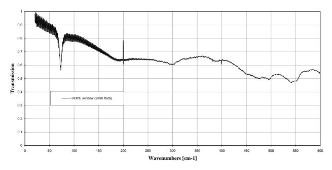
**Fig. C.2.** Measured transmission of a 2mm thick HDPE window from  $20 \text{cm}^{-1}$  to  $600 \text{cm}^{-1}$ . The polyethylene characteristic absorption increase is clearly seen around  $73 \text{cm}^{-1}$ .
