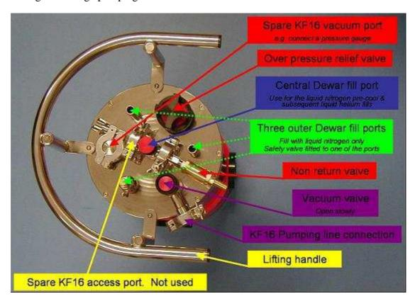
**Photo 2.1.** TK1813 cryostat top-plate fittings
