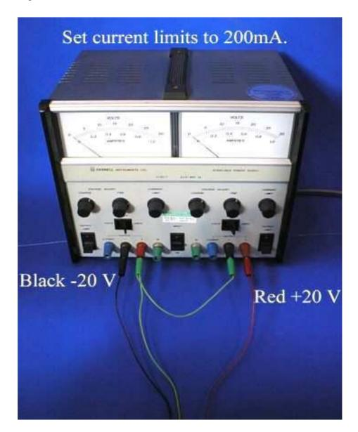
**Photo 5.2.** Power supply connections
