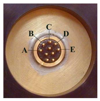
Photo 4.4. Electrical port pin assignments. Detector attached to pins B-E
