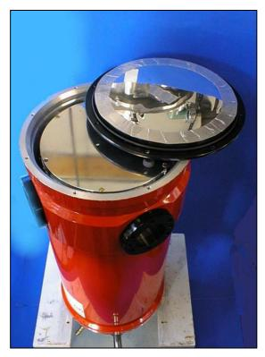
**Photo 1.4.** Liquid nitrogen base-plate in position
