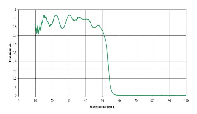
Fig C.1. Transmission spectrum for the 55cm<sup>-1</sup> low pass multi-mesh filter
