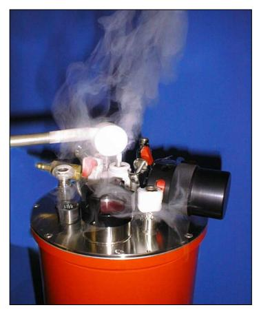
Photo 4.2. Helium gas exhaust during fill
